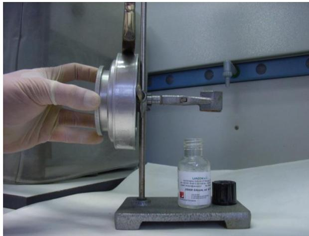
A 336 mm transparent Melinex® film strip is wound around a 107 mm diameter drum. The film is covered with a thin layer of 3% silicon fluid in carbon tetrachloride. The drum rotates by 2 mm/hr., allowing to sample without interruption up to 7 consecutive days without changing the sampling strip.
