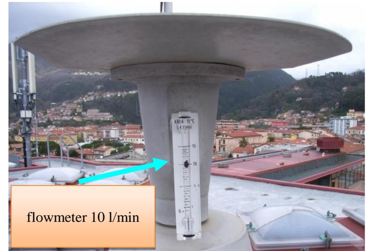
Suction pump ensures a constant air flow matching the respiratory flow, of 10 l/min (14,4 m<sup>3</sup> in 24 h). The trap has a range of 10 km, allowing a full coverage of the urban area.
